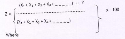
Y is the reading of the common energy meter installed on the 220 KV side of the Pooling Substation,  $X_{1,} X_{2}, X_{3}, X_{4}$  etc. are the readings of the energy meters installed at the various individual Wind power projects being developed/proposed to be set up in the area and connected to the Pooling Substation.
